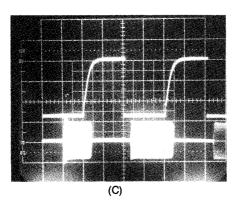
Fig 3—CW keying waveforms for the Kenwood TS-140S. The photo at A shows the keying waveform in the semi-break-in mode, and the photograph at B shows the keying waveform in the full-break-in (QSK) mode. In each photograph, the lower trace is the RF envelope; the upper trace is the actual key closure. Each horizontal division is 10 ms. The photo at C shows shortening of the first dot during semi-break-in operation. In this photograph, each horizontal division is 20 ms.
